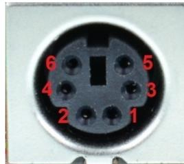
Figure 4: Mini Din 6 Female connector pinout
