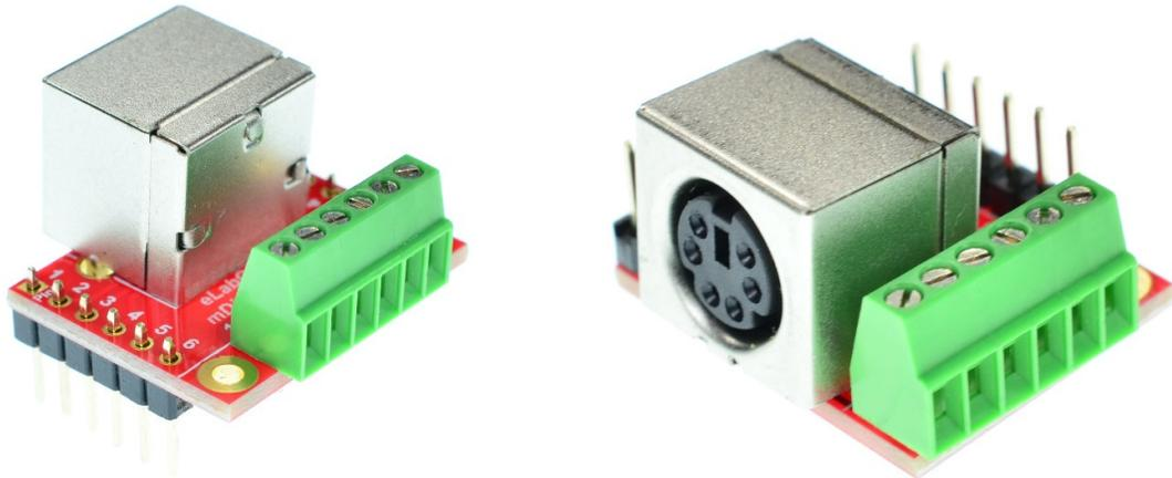
Figure 3: mDIN6-F-BO-V2A various connections
